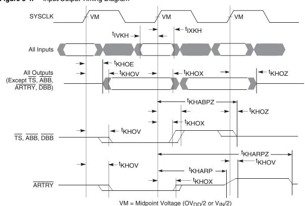
Figure 8-4 provides the input/output timing diagram for the PC755.
