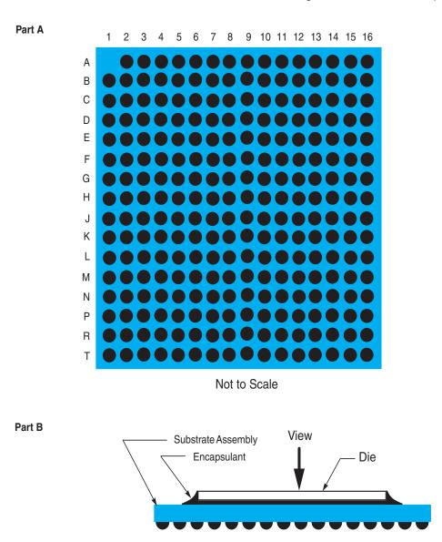
Figure 2-2 (in part A) shows the pinout of the PC755, 360 PBGA packages as viewed from the top surface. Part B shows the side profile of the PBGA package to indicate the direction of the top surface view.
