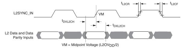
Figure 8-7 shows the L2 bus output timing diagrams for the PC755.
