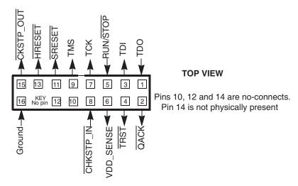
There is no standardized way to number the COP header shown in Figure 8-15; consequently, many different pin numbers have been observed from emulator vendors. Some are numbered top-to-bottom then left-to-right, while others use left-to-right then top-to-bottom, while still others number the pins counter clockwise from pin one (as with an IC). Regardless of the numbering, the signal placement recommended in Figure 8-15 is common to all known emulators.
