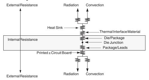
Note the internal versus external package resistance.
