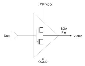
Table 10-1 summarizes the signal impedance results. The driver impedance values were characterized at 0°C, 65°C, and 105°C. The impedance increases with junction temperature and is relatively unaffected by bus voltage.
