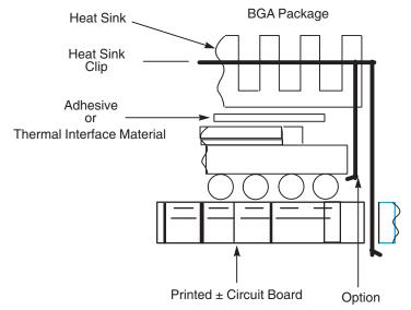
Ultimately, the final selection of an appropriate heat sink depends on many factors, such as thermal performance at a given air velocity, spatial volume, mass, attachment method, assembly, and cost.
