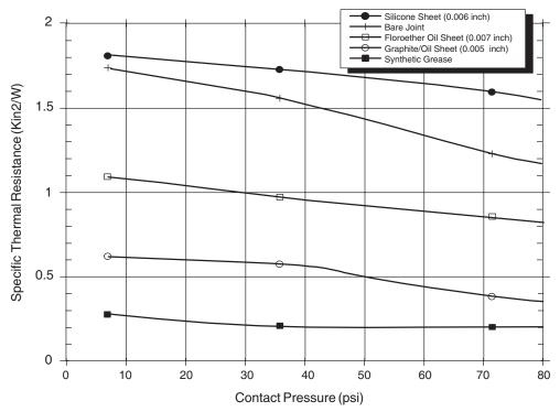
Figure 6-3. Thermal Performance of Select Thermal Interface Material
